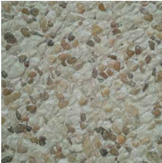
White stones 4 and brown stones 2, 3-6mm with white cement
