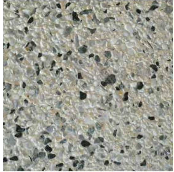
Calrrico and Verde Alpi stones with white cement
