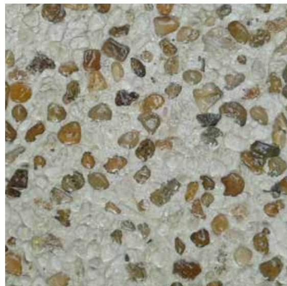
Brown stones 3-6mm with white stones 1-3mm with white cement
