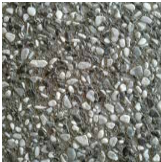
Bardiglio 4 and Calrrico 2 stones, 1-3mm with black cement
